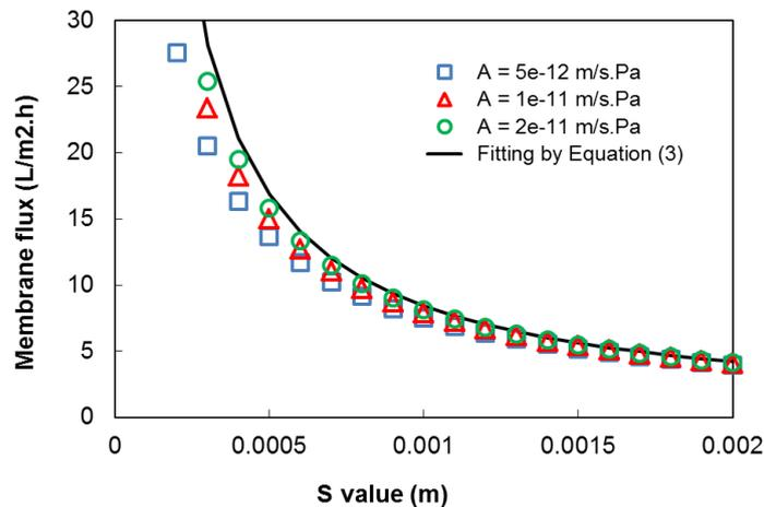
Figure 3: Effect of structural parameter ( $S$  value) on FO water flux for the seawater desalination scenario. Other simulation conditions include  $B/A = 10$  kPa and  $D = 1.69 \times 10^{-9}$  m<sup>2</sup>/s.
